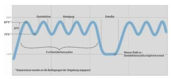
During the thermal disinfection the MoveoSiphon heats up to set temperature which is max. 95°C/203°F.
